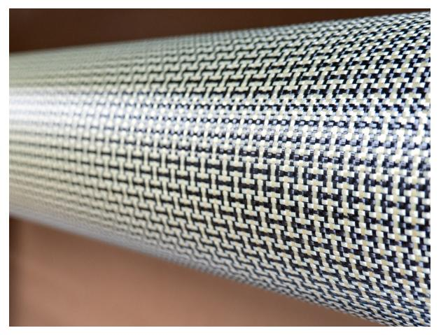
**Pros:** Combined Properties, Hybrid fabrics, like carbon-Kevlar<sup>®</sup> mixes, combine the benefits of different materials, offering both strength and impact resistance.
