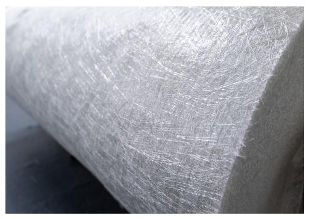
**Pros:** Easy to Use: Metycore is designed to conform easily to shapes, making it ideal for complex closed moulds, resin infusion and vacuum bagging.
