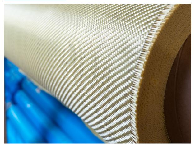
**Pros:** Great impact resistance, superior tensile strength, lightweight. The tensile strength of Kevlar<sup>®</sup> is over eight times greater than that of steel of equal weight. It also withstands the extremes of temperature as well as the effects of salt water and other natural occurring chemicals.
