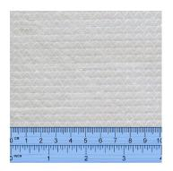
**Pros:** Multidirectional Strength: Features fibres running in three directions, providing strength and stiffness in multiple axes.
