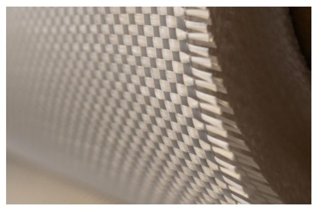
**Pros:** High Impact Resistance: Diolen offers excellent resistance to impact, making it suitable for products requiring high durability. It is also more economically priced than that of Kevlar<sup>®</sup> if you want high impact resistance without abrasion resistance.
