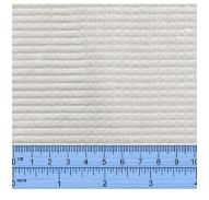
**Pros:** Multiaxial Strength: Combines fibres in four directions, offering excellent strength and stiffness in various orientations.
