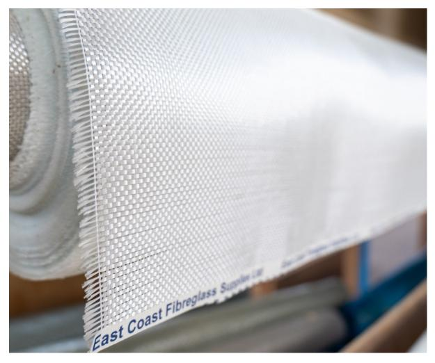
**Pros:** Affordable, versatile, compatible with various resins. Available in very light weight options such as 25g and 28g which are ideal for model aircraft etc and up to 200g, which is excellent for sheathing plywood canoes and kayaks when combined with an epoxy resin. Also available in rolls of matting, these are randomly laid 2" cut strands held together with a binder, an emulsion binder for Polyesters/Vinylesters and a Powder bound version for Epoxy Resins.
